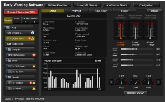
Temperature, lamp usage hours, and fan voltage meters
